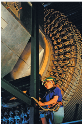
Blocking Materials separate and stabilize coil ends and phase leads in power generators.
