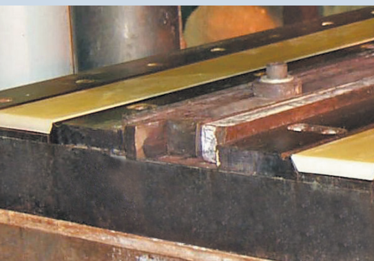
Molded and Machined Wedges can withstand extreme compressive force at high temperatures.
